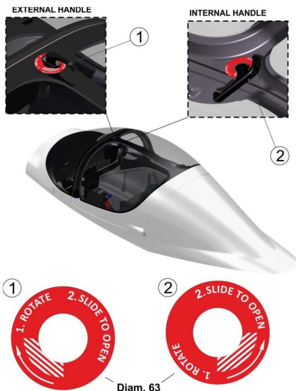
Figure 7-5 – Canopy Door Opening
