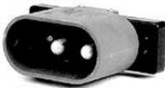
Figure 7-14 - External power Receptacle
