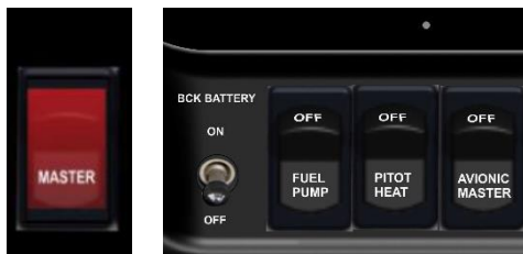
Figure 7-13 - Electrical Main Switches
