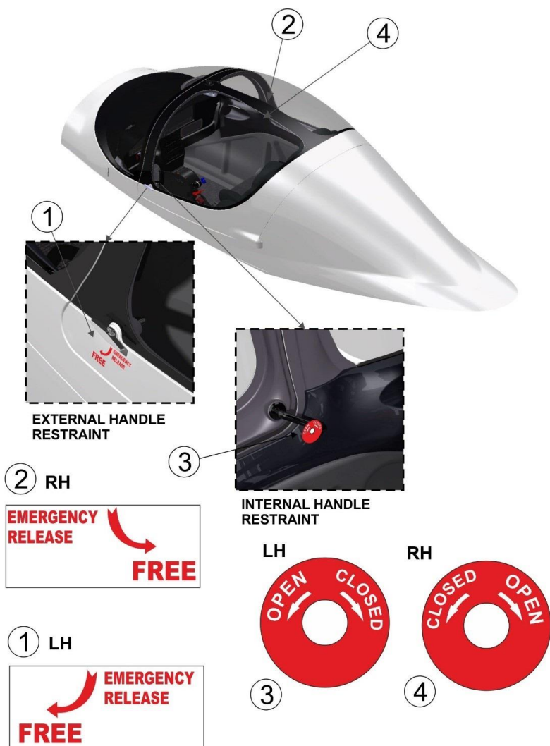
Figure 7-38 – Emergency Exit Placard
