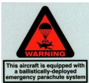
Figure 7-47 – Parachute Entry areas warning placard
